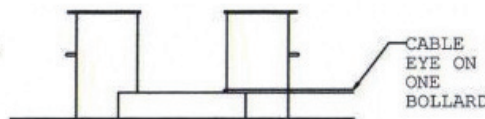
FIGURE B (CABLE LOAD = 2 SWL) CABLE END EYE POSITIONED ON ONE BOLLARD ONLY :CABLE LOAD=2 SWL
